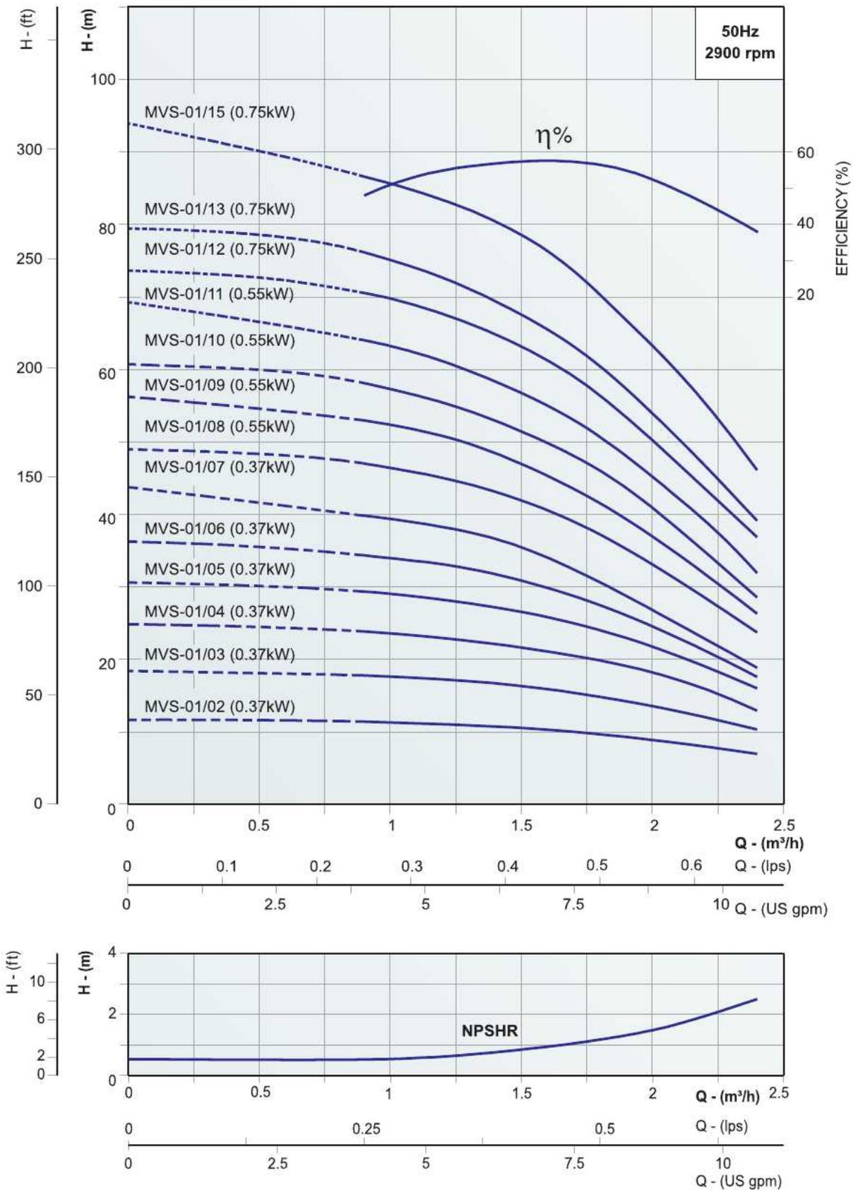
Replace the 3rd digit in model name as "C" for Cast Iron pump base & pump head models and "N" for SS 316 construction.
